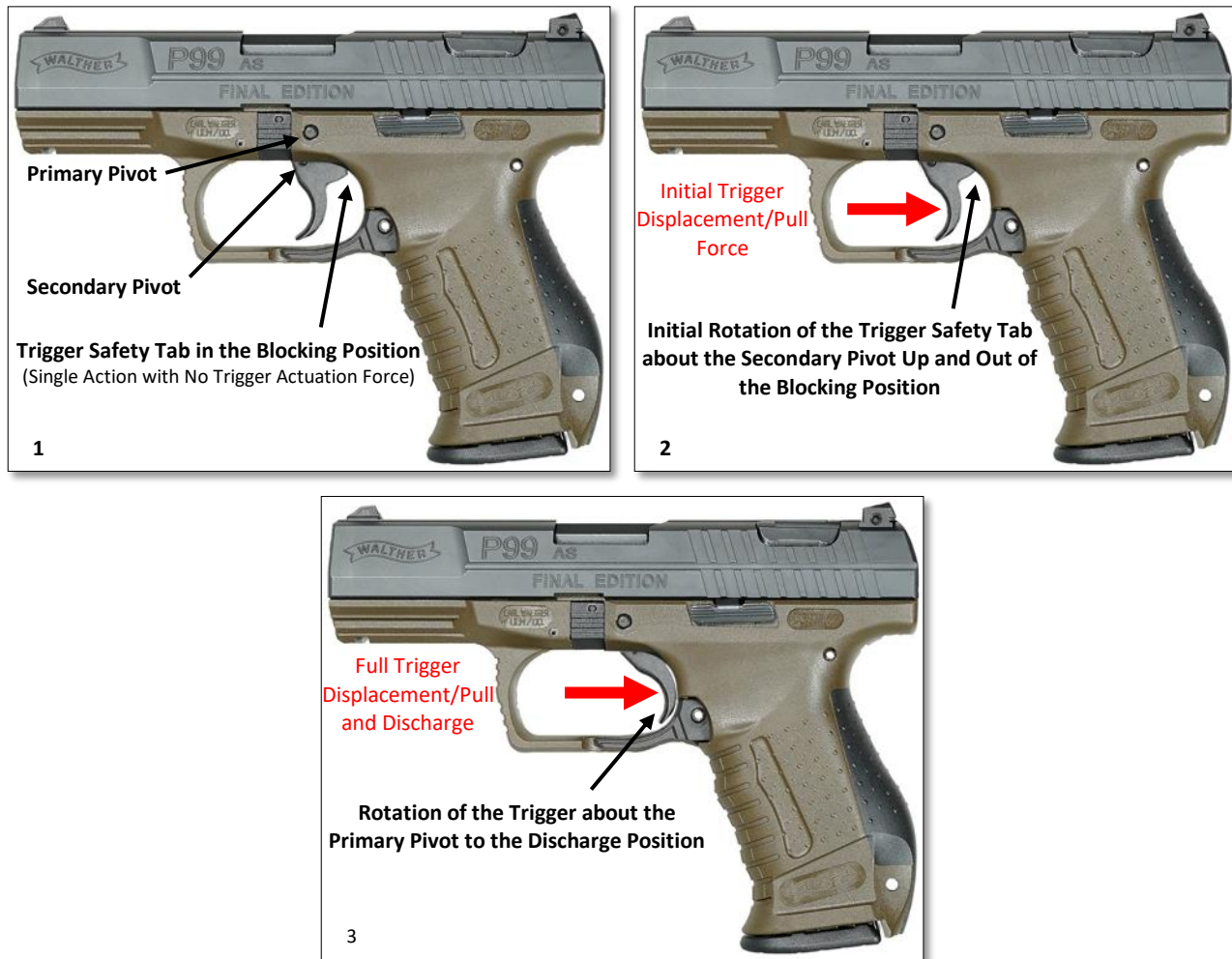
Figure 5.3.6: Functionality of a Walther P99 Passive Articulating Trigger Safety in Single Action Mode (100% Cocked)
