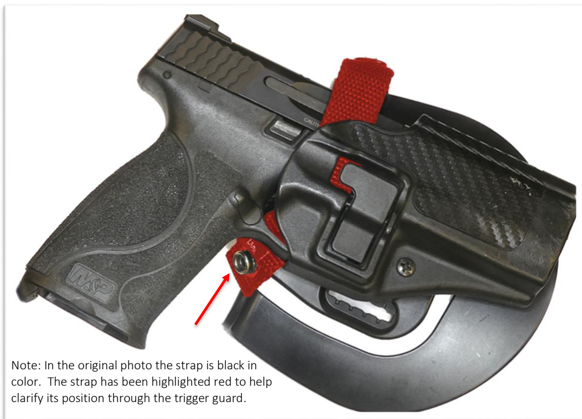
Figure 7.3.7: Actuation of a Trigger Equipped with a Trigger Safety, Caused by a foreign Object in the Holster
